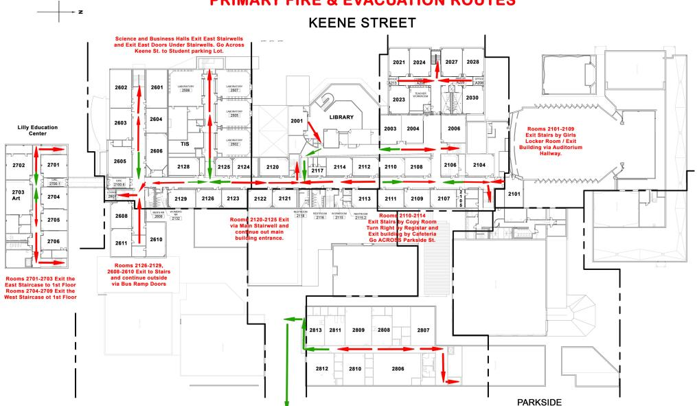
SECONDARY ROUTES: Green Arrows indicate alternate routes. These routes are ONLY to be followed if Primary Escapre Route is blocked by fire of debris.
